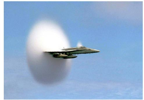
A jet aircraft "breaking the sound barrier" - traveling faster than 343 m/s.
