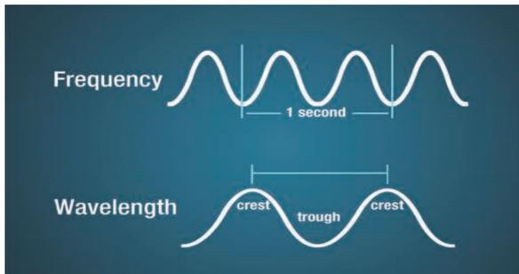
When you look at a representation of a simple [sound wave](#) (let's say the note "C") on an oscilloscope or another visualization tool, you will see a squiggly line going up and down in a regular pattern. This pattern, the [sound wave](#), contains three attributes: wavelength, [frequency](#), and [amplitude](#).
